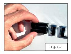
**6.** Lightly press down to adhere overlay to the factory emblem. (Fig C-6)
