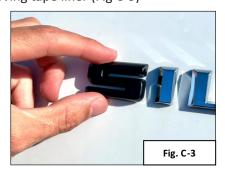
**4.** Use pull tab to remove adhesive liner from backside of overlay. (Fig C-4)
