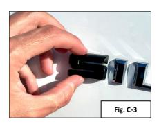
**4.** Lightly press down to adhere overlay to the factory emblem. (Fig C-4)
